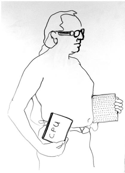
Figure 2: Early sensory substitution device. Camera attached to the eyeglasses transmits to a needle array on the belly. Graphic by the author, after Bach-y-Rita (1972). Reproduced with permission of Elsevier Publisher, UK.
